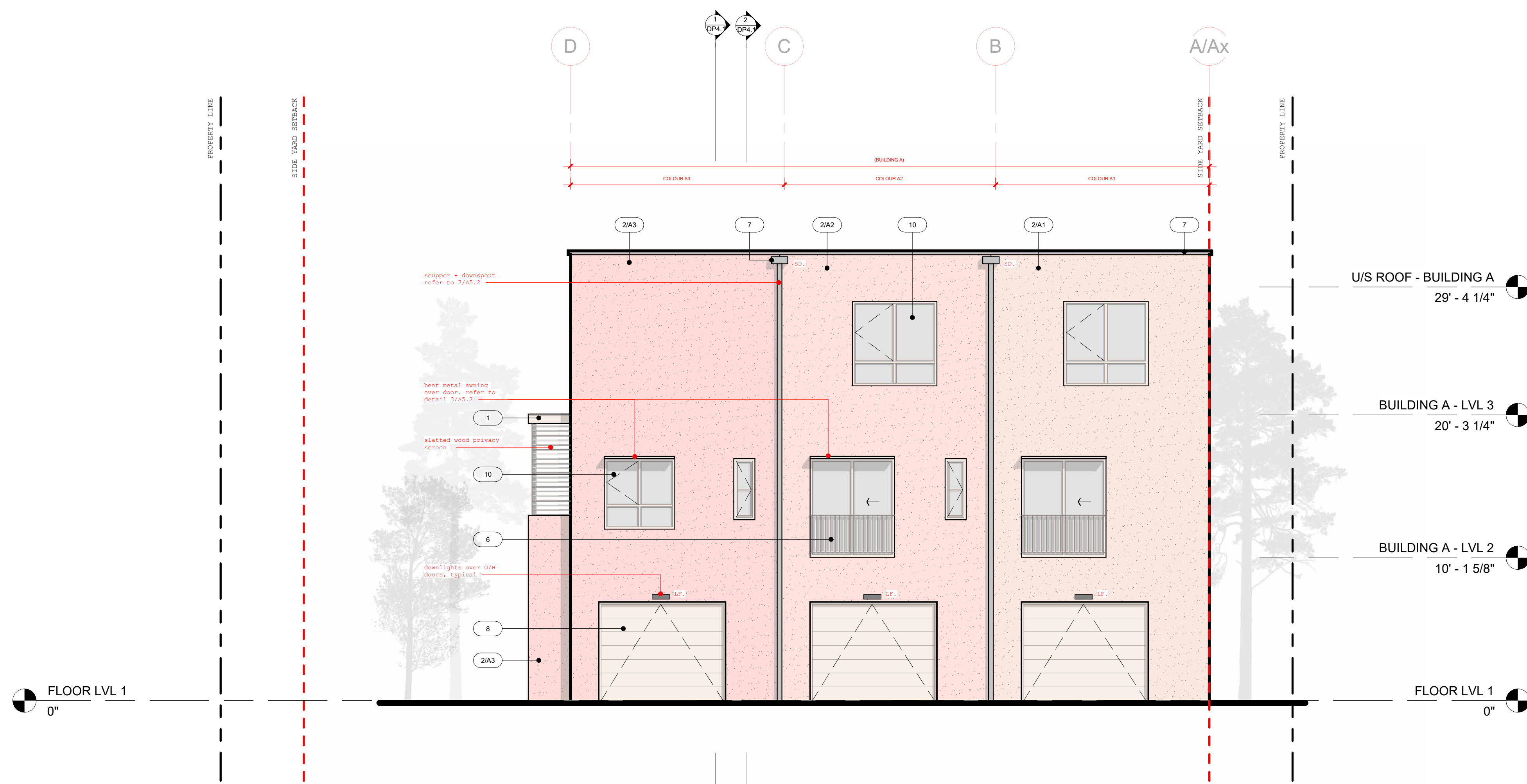
1 BUILDING A - EAST ELEVATION - DP 3/16" = 1'-0"
